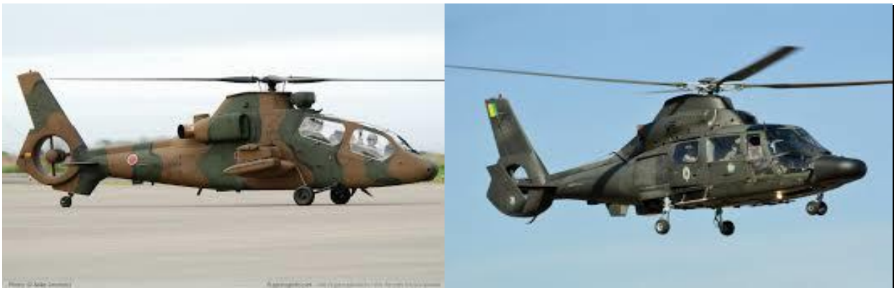
řekil 25: Fenestron Kuyruk Rotoru Kullanan OH-1 Ninja ve AS 565 Panther
